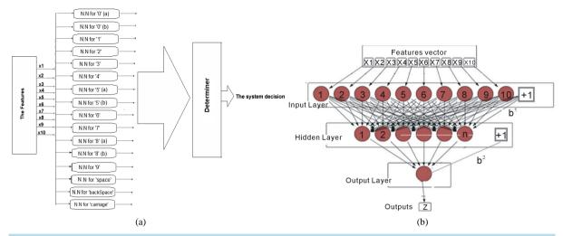
Figure 5. (a) Block diagram of PNN classifier; (b) one of neural networks of PNN classifier.
