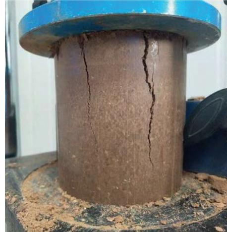
FIGURE 4: Photograph of an unconfined compressive strength test.
