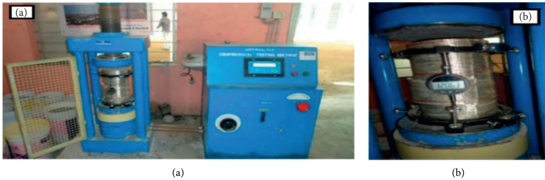
FIGURE 10: (a) Arrangement of experimental set. (b) Testing of GFRP-wrapped columns in compression testing machine.
