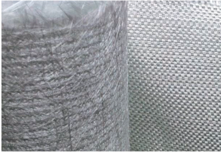
FIGURE 5: Woven roving Combi mat laminated sheet.
