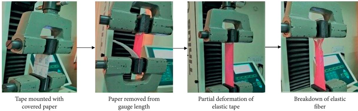
FIGURE 3: Three steps of sample mounting for a tensile test of tapes. (a) The tape is mounted with covered paper. (b) The paper is removed from gauge length. (c, d) The test is run up to failure.
