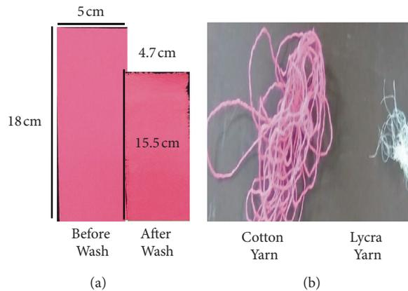
FIGURE 6: (a) Tape after wash and before wash. (b) Cotton and lycra yarn.
