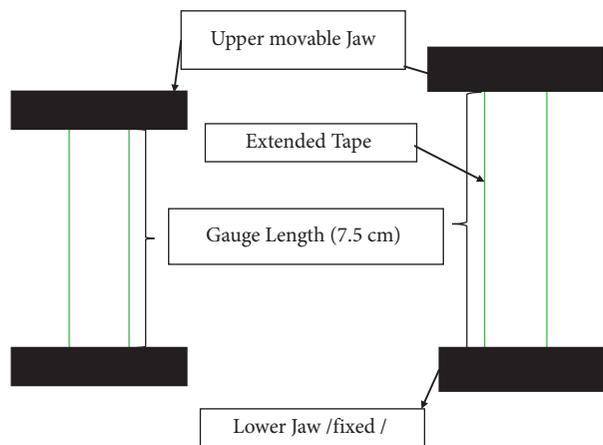
FIGURE 4: Method of the stress relaxation test under 25% and 50% level of extension.
