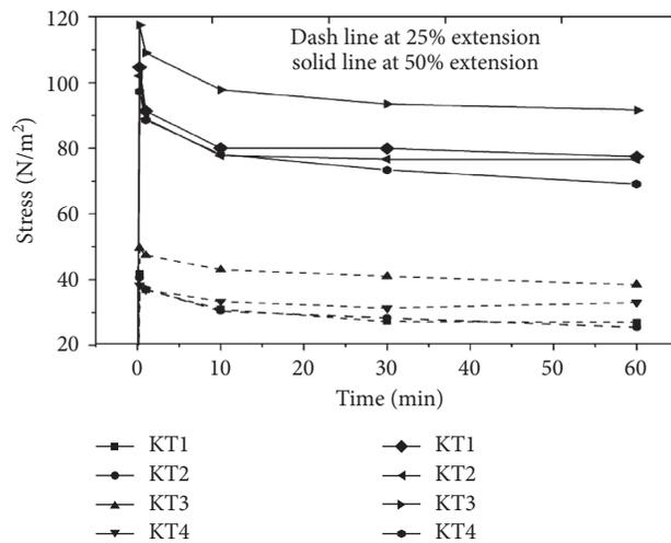
FIGURE 8: Stress response of the therapeutic tape under two levels of extension.
