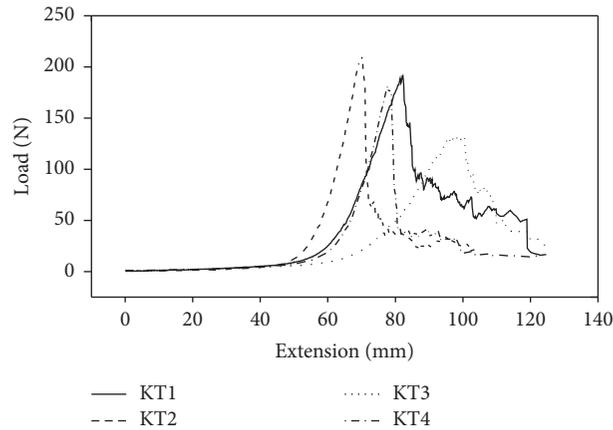
FIGURE 7: Tensile characteristics of each tape.
