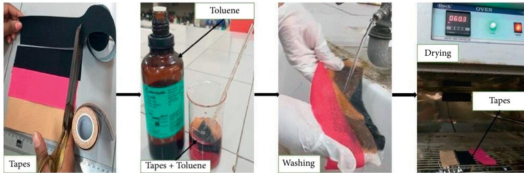
FIGURE 2: Process of adhesive removal from each tape.
