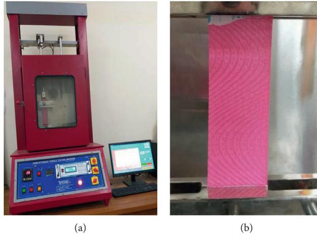
FIGURE 5: (a) Tensile testing machine with the heating chamber and (b) sample mounting position.
