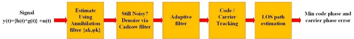
Figure 3. Overall view of the proposed block diagram.
