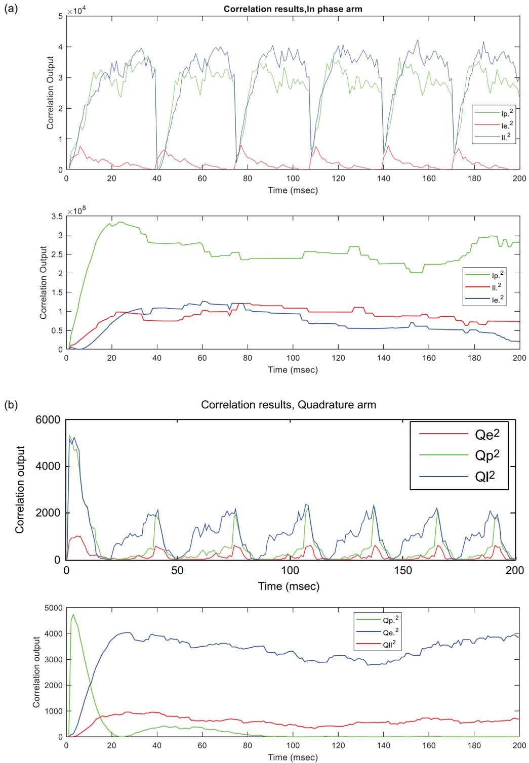
**Figure 13.** (a) Correlation results of in-phase arm before and after applying to the annihilation filter. (b) Correlation results of the quadrature-phase arm before applying to the annihilation filter.
