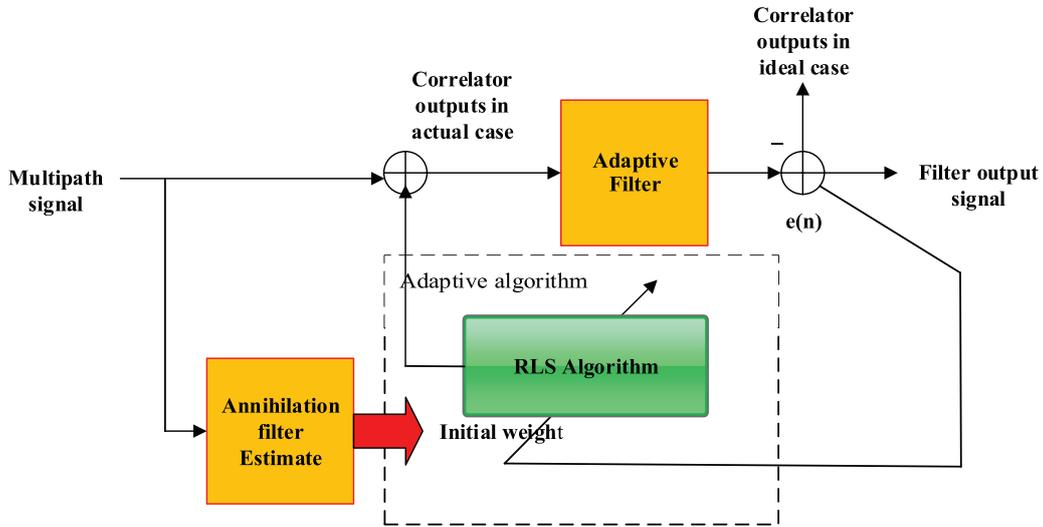
**Figure 5.** Estimation of multipath parameters via annihilation filter combined adaptive filter.
