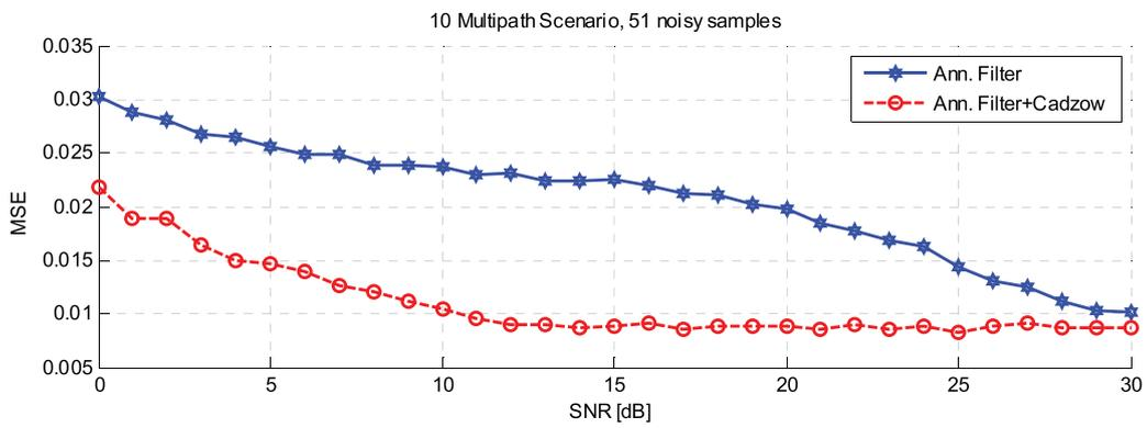
Figure 10. Comparison of SNR versus MSE with LP = 10 and N = 51, with and without cadzow algorithm.
