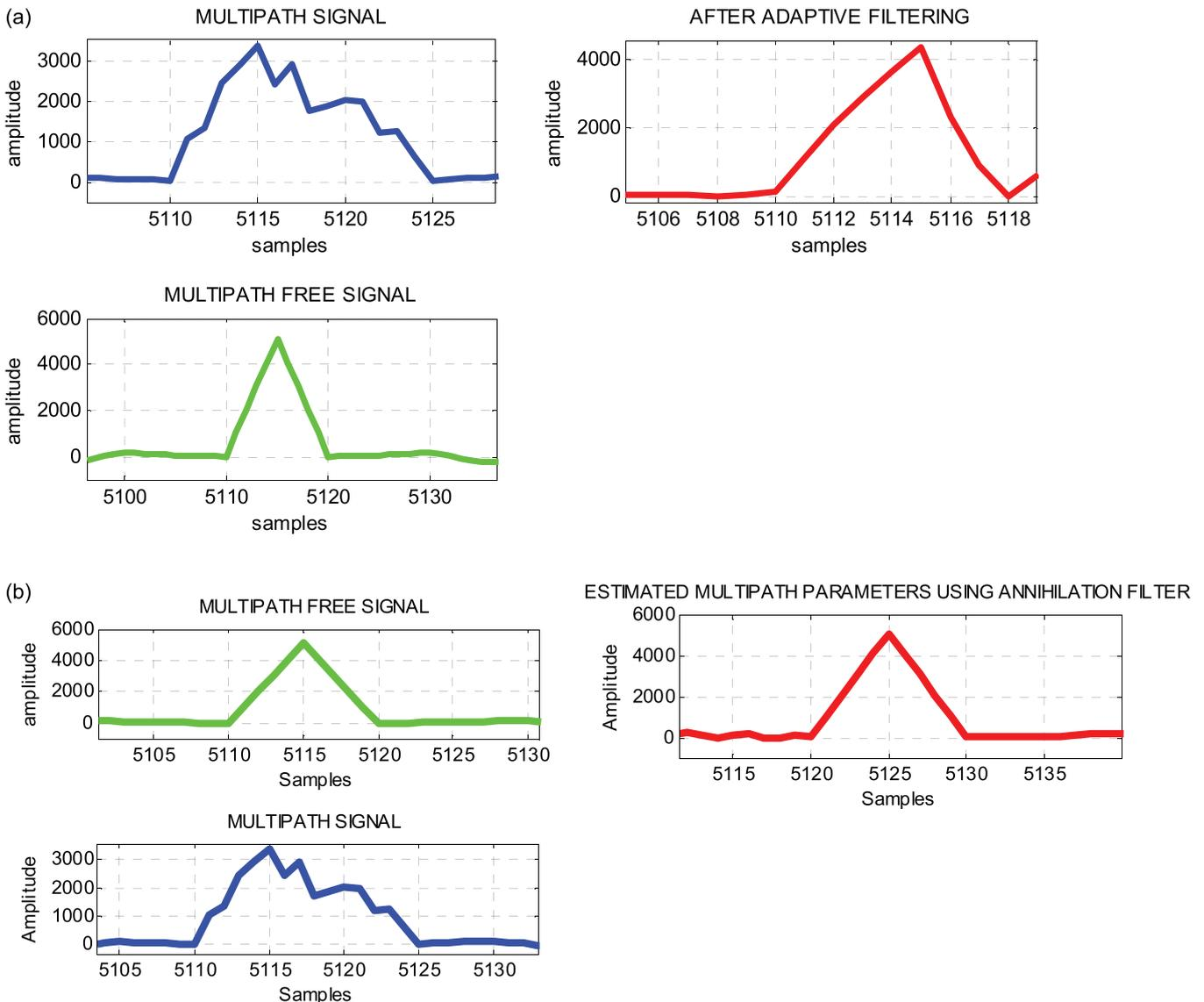
**Figure 12.** (a) Correlation results of least-square based estimation used in adaptive filters. (b) Correlation results of annihilation filter-based parameter estimation used in adaptive filters.
