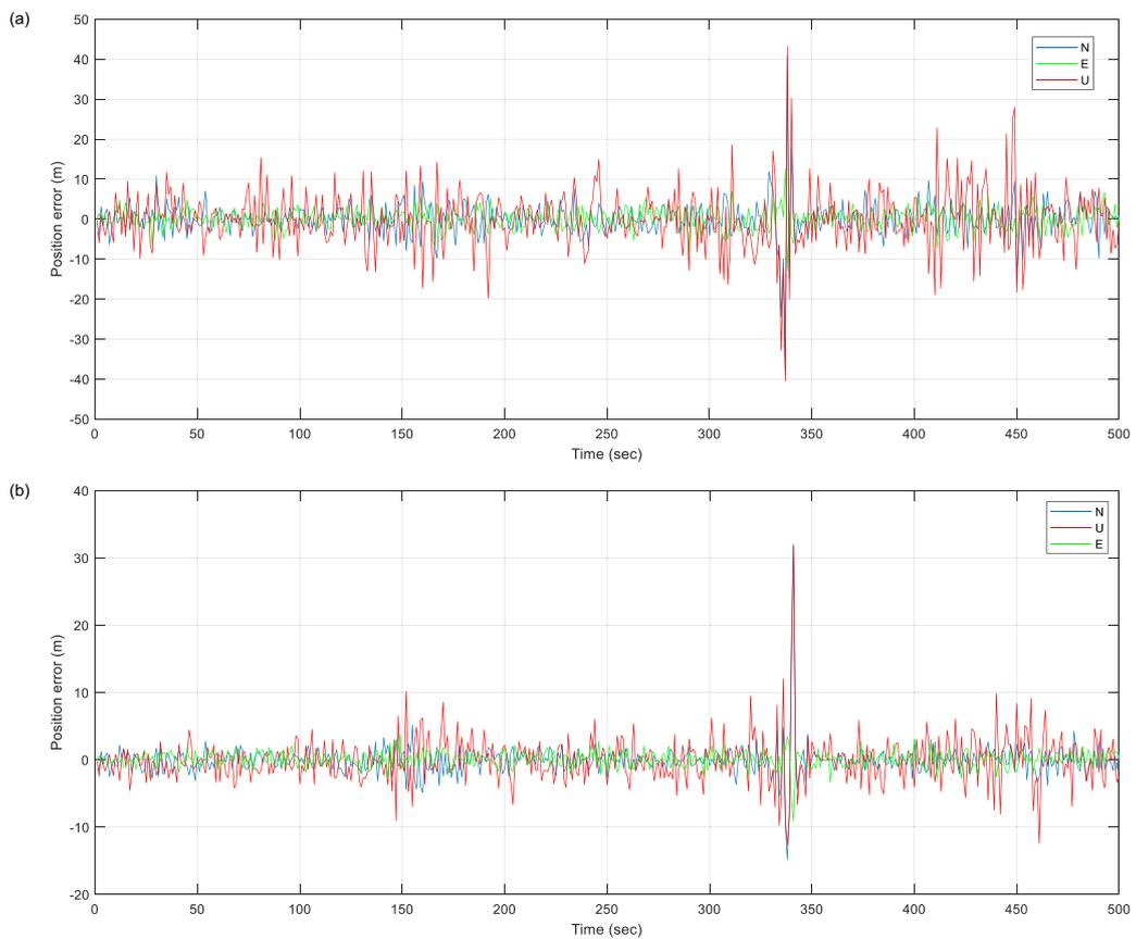
Figure 17. Positioning error computation. (a) Without annihilation filter. (b) After inserting annihilation filter in the tracking loop.
