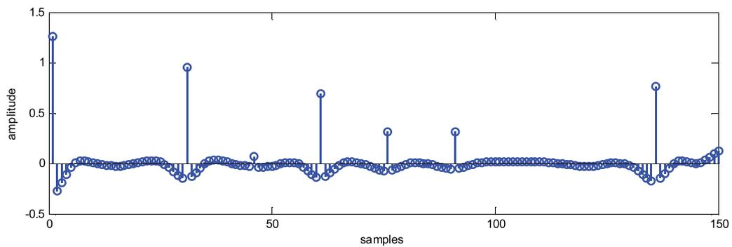
Figure 11. Impulse response of an inverse filter/adaptive filter.
